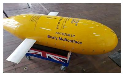
Boaty McBoatface is a small 3 meter (~10 ft) Autonomous Underwater Vehicle. It can be programmed by the science team to go and collect data, diving to depths of 6000 meters (3.7 miles) and under an ice shelf!
