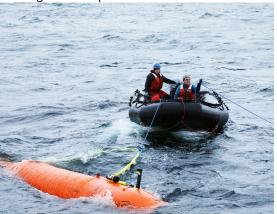
After *Ran* safely resurfaces members of the team are sent out in an inflatable zodiac boat to 'catch' it and pull it back to the ship.
