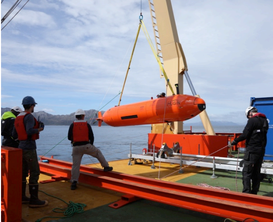
The team sends Ran down ~0.5 miles (1 km) under 1000-1500 ft. (300-500 meter) thick floating Thwaites' ice to map the sea bed, collect water samples & measure circulation.
