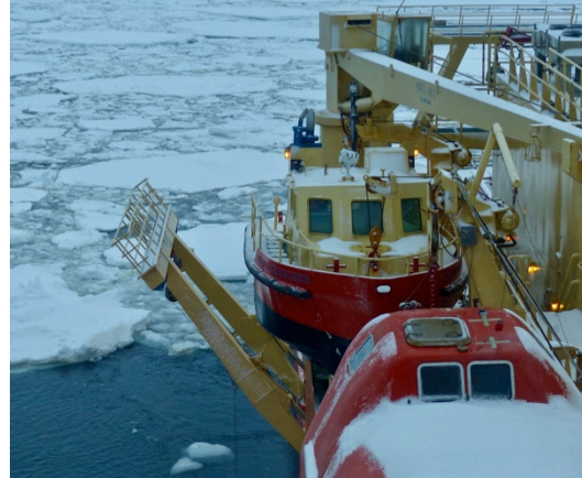
The research ship suspends an instrument in the ocean to communicate with the Hugin while it works underwater so it doesn't try to resurface under shifting sea ice conditions.
