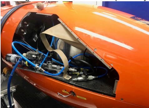
Hugin's control center and the CO bladder used for floatation in this ~15 ft. (4.5 m) submarine.
